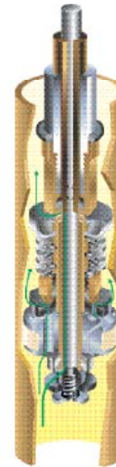
INTERMEDIATE HIT Low-speed port open Shim stack open
